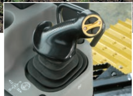
PCCS-Bedienhebel (Palm Command Control System)
